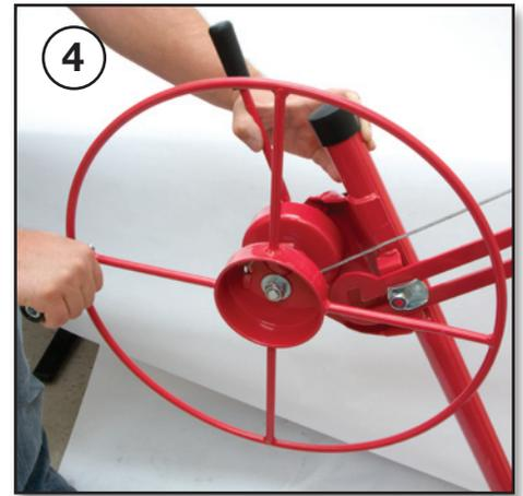
5. Press the winch assembly slightly back toward the frame.
